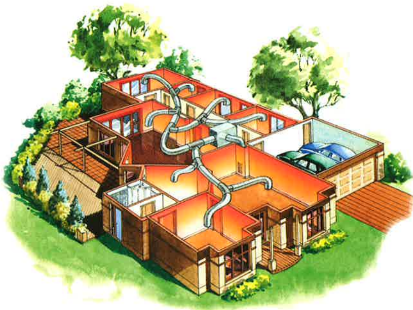
Typical unit and ducting layout of a roof space mounted internal unit installation. *Installer set.
