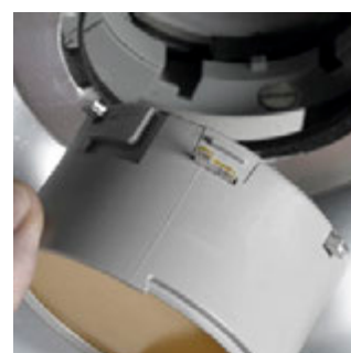
LED module includes ballast and can easily be changed using the bayonet mount.
